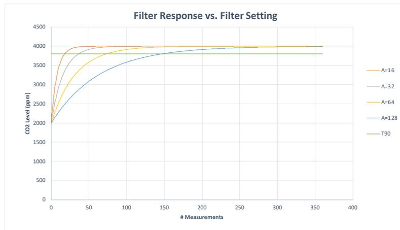
The graph above shows the effect of the filter on response times. Increasing the filter setting increases the measurement output response time. T<sub>90</sub> is the time to 90% of reading. The ExplorIR®-M takes 2 readings per second.
